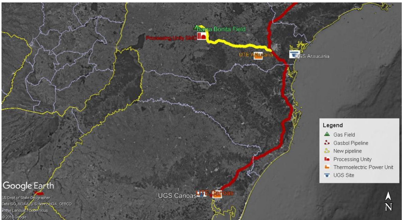
Figure 21: SMO-Araucária pipeline and possible locations for UGS sites: Araucária (PR) and Canoas
